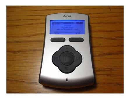
DONE. Your new antenna is invisibly hidden inside the housing and will boost the transmit range from about 3-4 feet to about 50 feet.
