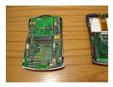
Flip the main board over and place it in the back part of the housing, so the front is facing up, as shown.
