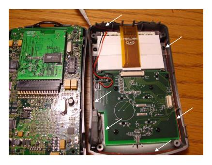
Carefully run the wire using a pair of tweezers or needle-nosed pliers around the housing as shown. The longer the wire is, the better.
