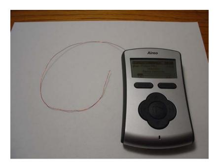
Now the Aireo has an external antenna for transmission. This allows an incredible transmission range boost. The longer the wire, the stronger the radiation. The optimal length is 1 Meter (~3 ft.) which acts as a quarter wavelength antenna with best efficiency. 1 ft. Usually is more than enough to receive your Aireo's signal throughout a whole house.
