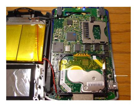
Place the main board back into place and make sure the white connector is put back in place. After that you must press the marked RESET button once to reboot the player. Otherwise the LCD will stay blank. Close the housing and screw the four screws back in.
