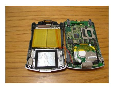
Carefully flip the back of the player open. Pay attention to the wires! There is a wire to the Wi-Fi antenna and two wires to the battery.
