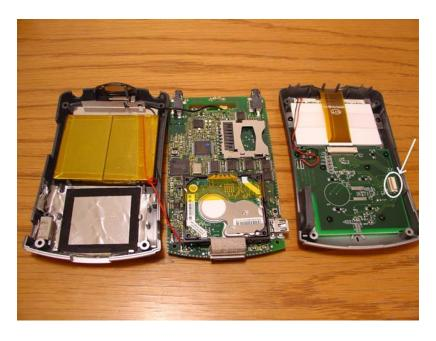
Take the main board out of the front part of the housing by carefully pulling it off the maked white connector.
