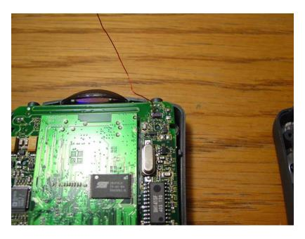
For maximum POWER, solder the wire to L1 and run it to the left headphone socket.
