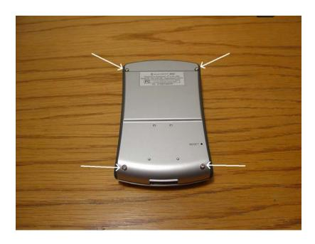
Remove the four screws as shown with the screwdriver
