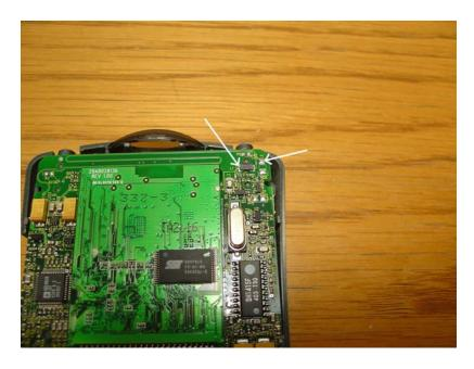
Locate the marked soldering spots. They are labeled "L1" and "L2".
