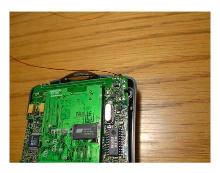
One way to improve the transmit range is to solder the wire to L2 (or L1) and place it inside the player's housing.
